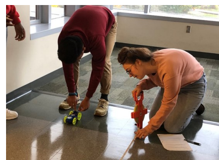
Ready, Set, Go—The solar cars efficiency is measured by seeing how far they go on a solar charge
