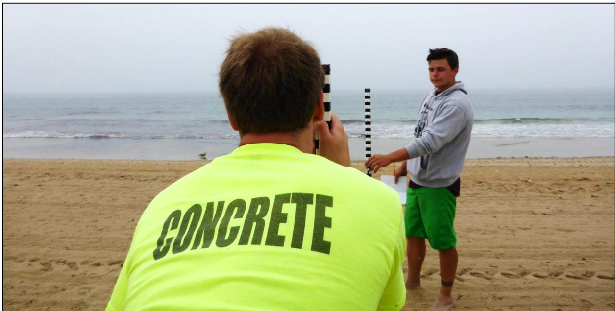
Environmental Earth Science majors Tim Ciskowski and Cody Murphy measuring beach profiles using the modified Emery (1960) method on Misquamicut State Beach, Westerly, RI: June 2015.
