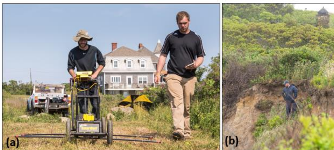
(a) EES students Tim Ciskowski (right) and Kevin Veilleux (left) collect 100 MHz GPR data across a sinkhole beside an access road and near (b) a large cliff on southern block island (supervisor B. Oakley for scale).
