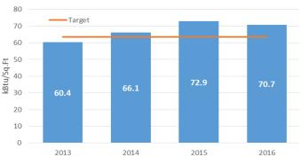
Figure 1. Building energy performance (site EUI) by calendar year from 2013 to 2016 (in blue) and a proposed energy use target (in orange) for Asnuntuck Community College. The target reflects a 10% reduction in energy use from 2016 use.
