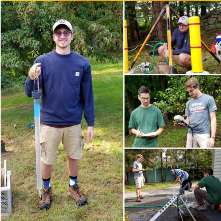
Bryce Mase (above) and Erick Bora (below) assisting in water quality sampling and profiling of fractured bedrock wells to better understanding salt contamination and fracture flow conditions.
