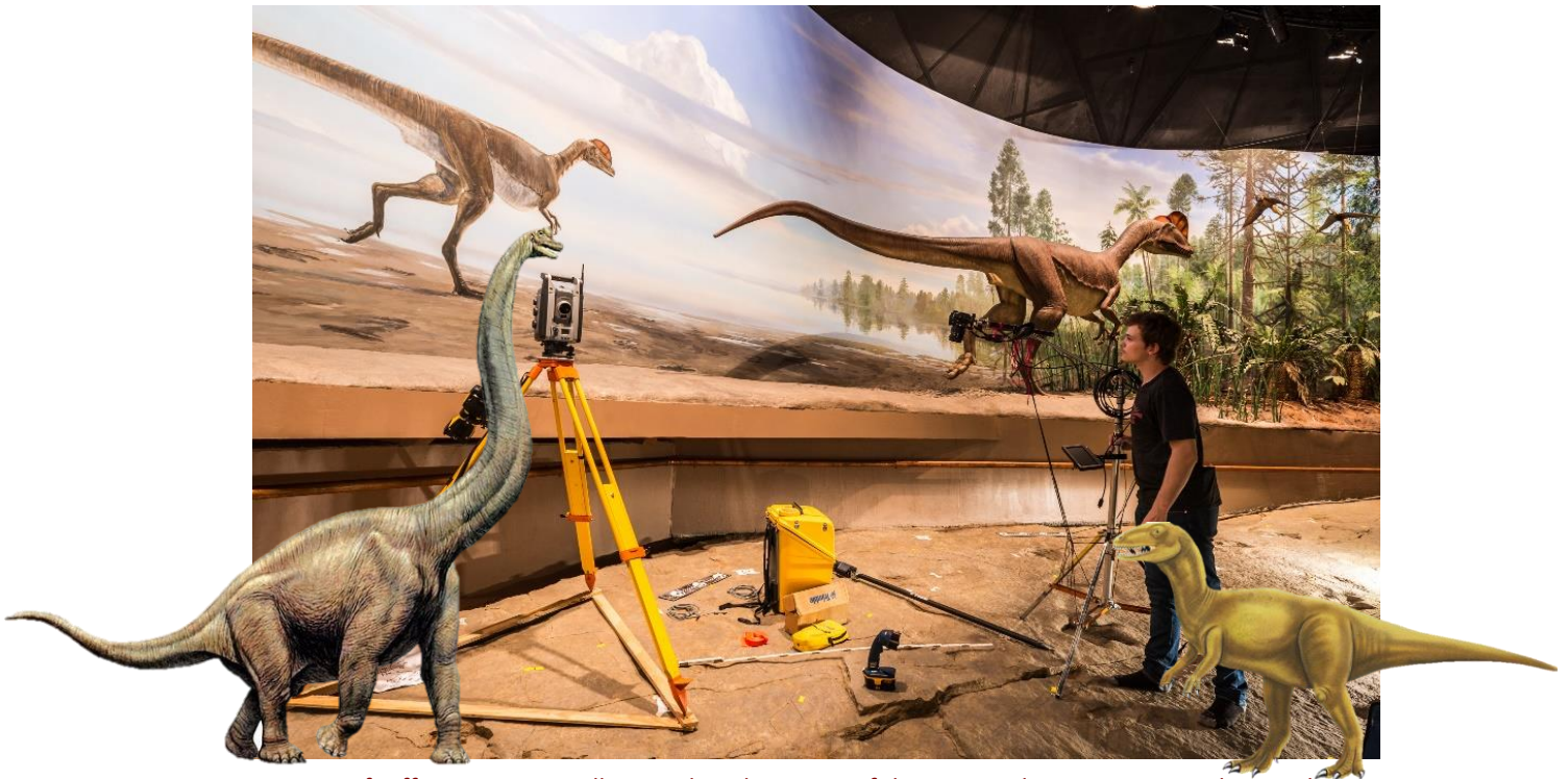
Image of Jeffrey Fontaine collecting digital imagery of the DSP tracksite using a sturdy tripod. Jeffrey and Ryan were also used laser surveying equipment in this image to measure location of photo-grammetric targets. PLUS some uninvited visitors.
