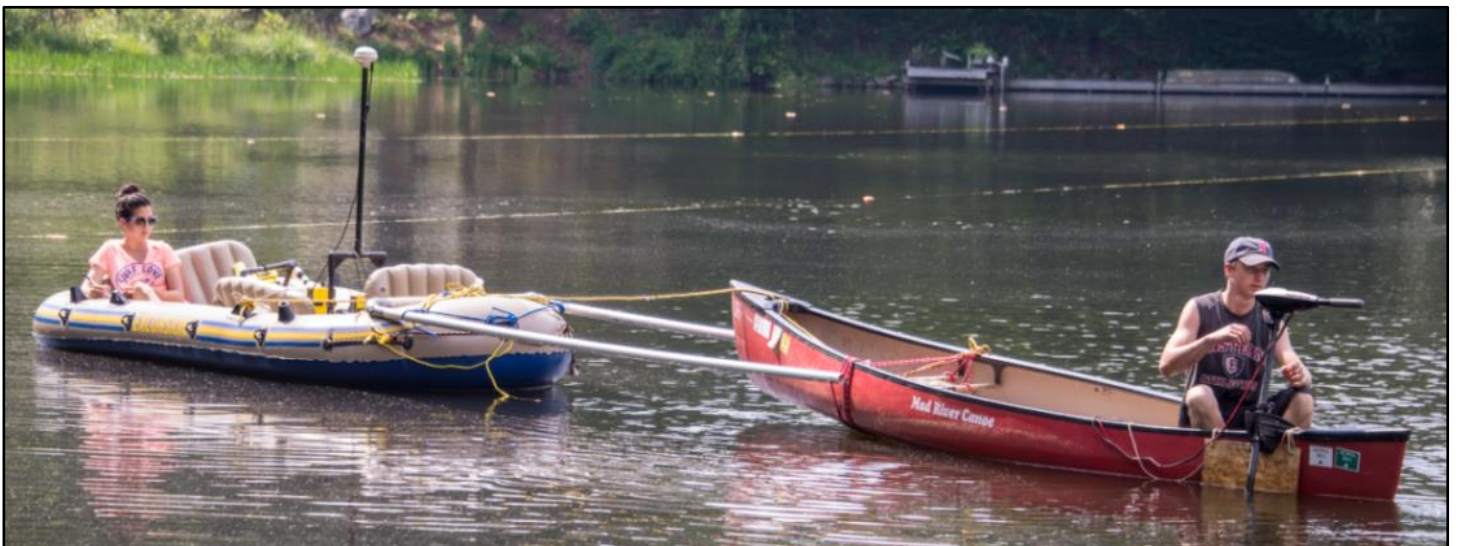
Ashley Hole (left) and Trent Stevens (right) prepare to collect ground penetrating radar data on Andover Lake. Trent is driving a pull boat (in reverse) while Ashley is managing controls on the GPR unit.
