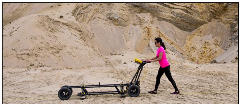
Ashley Houle collects 100 MHz GPR data on a transect at the Haines Sand and Gravel mine in Windham. She is learning to process these data to image subsurface geological conditions.
