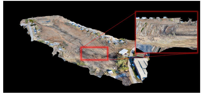
Figure 7. 3D model of the Arboretum created in Drone Deploy. While detail is realistic, the inset shows error associated with merging model data from two flights with differing take-off elevations. This can be addressed within DD softer, but is better resolved by using a single take-off location.
