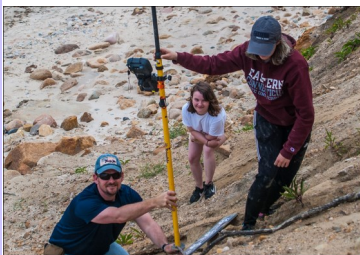
Figure 6. Gathering RTK GPS data on Block Island
