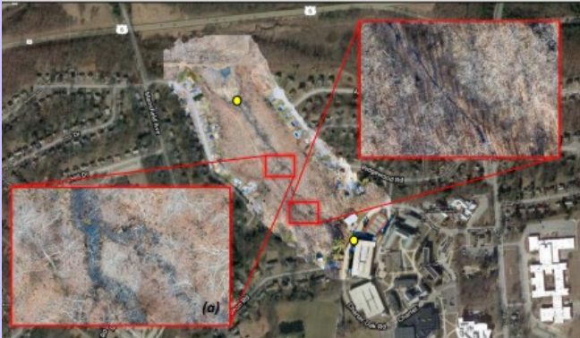
Figure 6. Aerial view of the Arboretum taken from the Drone Deploy website after uploading the 956 images captured with two flight lines at 90° to each other. Flights used 2 sets of parallel flight lines with 75% forward overlap and 80% forward and 75% side overlap. Insets show close views of (a) a stream section separated into two segments. A photogrammetric target can be viewed as well. Inset (b) shows a close-up view of a site from the upper flight. Note extensive shadows caused by sunny conditions during the flight. This upper-lower flight boundary causes elevation mismatches (see Fig. 7).
