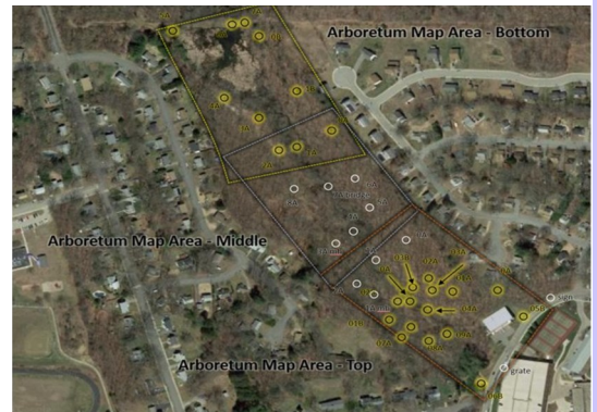
Figure 5. Map view of the Arboretum including photogrammetric target locations in yellow. The Arboretum was separated into 3 sub-sections for imaging to limit the distance the drone had to fly away from the operation.
