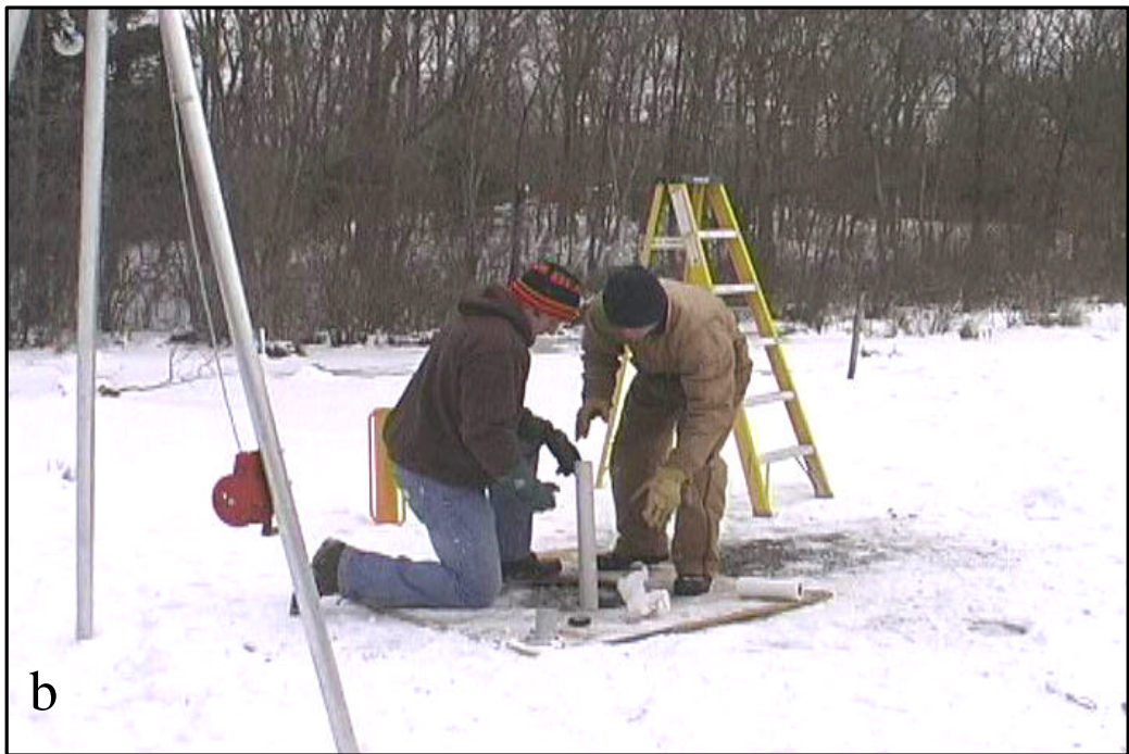
Figure 4: Photograph of coring apparatus including a) assembling the coring tripod and b) removing core through the platform.
