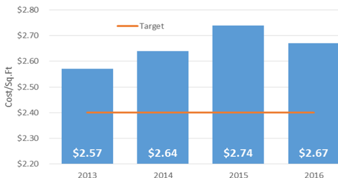
Figure 4. Energy cost per square foot for Capital Community College from 2013 to 2016 (in blue) and a proposed target (in orange) that assumes a 10% reduction in energy use.
