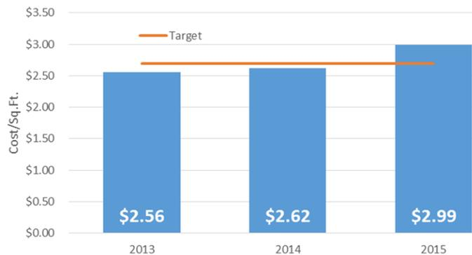
**Figure 4. Energy cost per square foot for Tunxis Community College from 2013 to 2015 (in blue) and a proposed target (in orange) that assumes a 10% reduction in energy use.**
