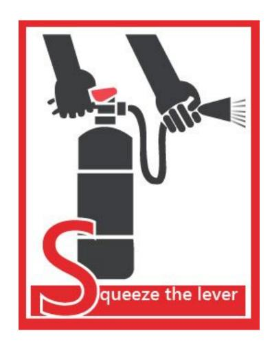
This depresses a button that releases the pressurized extinguishing agent in the extinguisher
